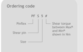
Select coupling based on nominal torque using service factors from page 13. Then select required shear torque from table below.
